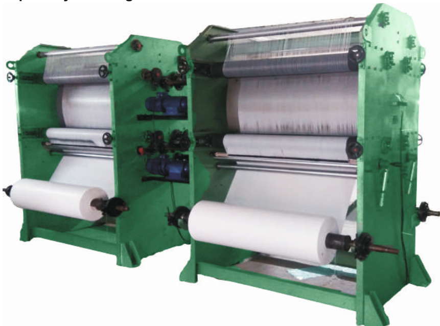
SG-130" High Speed Single-Bed Raschel, Mosquito Net & Cotton Net Machine
